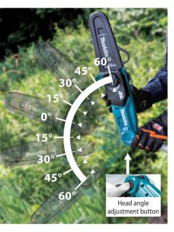
The angle of the tool head is adjustable in 9 stages between 60° upwards and 60° downwards.
